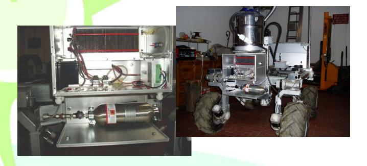
The figure above shows an application of robotics created by H2planet: This is a robot dedicated to the collection of saffron and other agricultural activities of various type: in this case the autonomy and the lack of polluting emissions were the determining factors in the selection of hydrogen technology.
